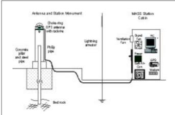
Fig. 2: Configuration of a MASS Station with Cylindrical Concrete Pillar
